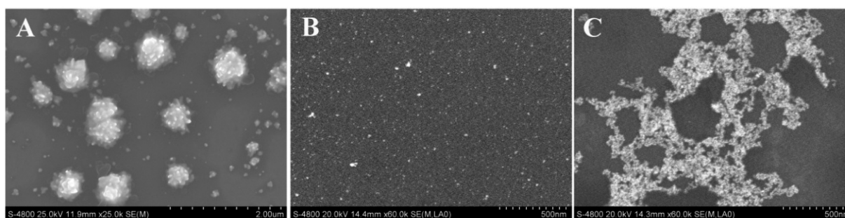
Figure 1. SEM images of (A) AuNFs, (B) PAMAM-Au and (C) Fc-Fc/ \beta -CD/PAMAM-Au.
